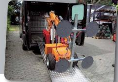
The Smartlift is easily transported in a van or on a trailer
